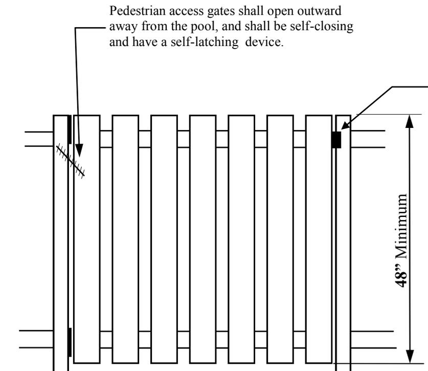
The latching device must be located at least 48" above the bottom of the access gate.
