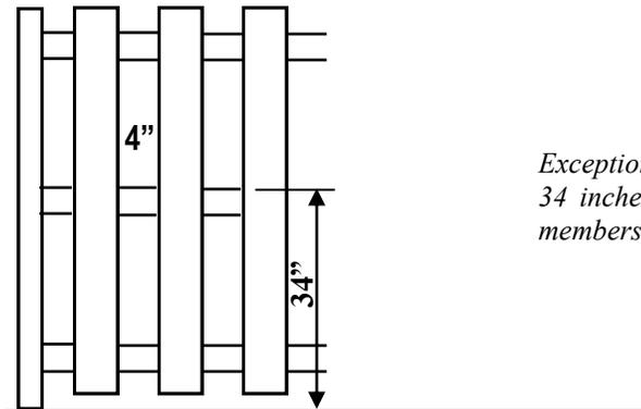
*Exception: When intermediate horizontal members are located 34 inches or more above grade, the spacing between vertical members shall not exceed 4 inches in width.*
